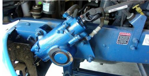
GEAR WITH BLEEDER PLUG - SECTOR BORE ABOVE PISTON
